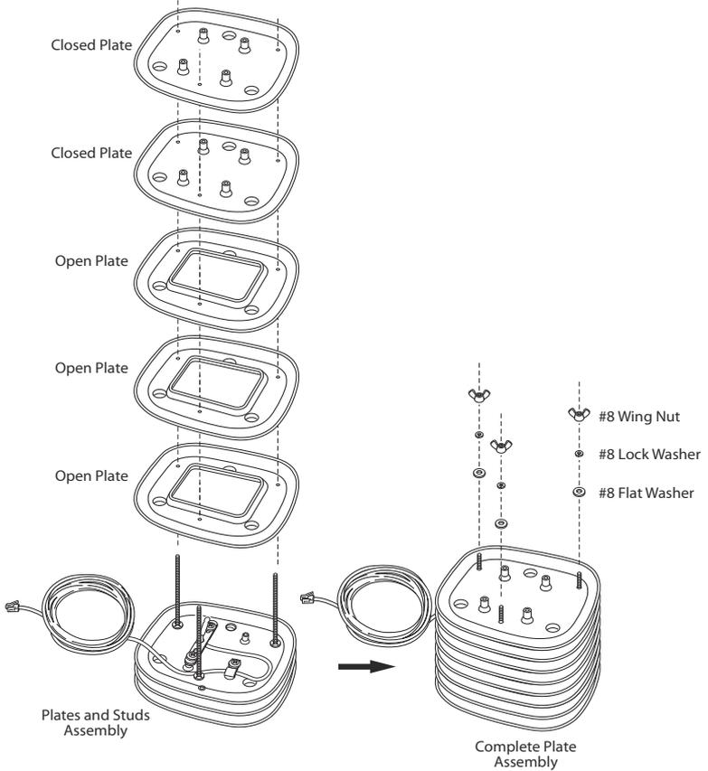
2. Place the flat washers, lock washers and plastic wing nuts over the protruding stud ends.
