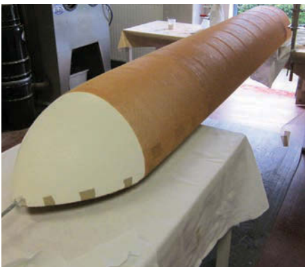
The Litus fuselage under construction showing the honeycomb material as part of the skin
