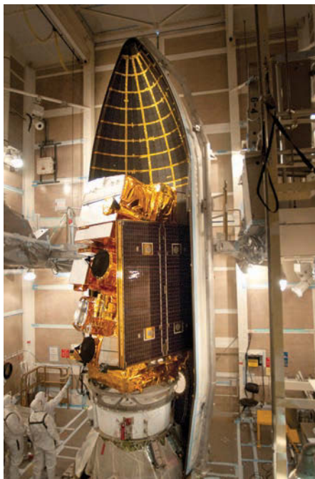
The S-NPP spacecraft is installed in its rocket housing, a United Launch Alliance Delta II-7920-10 launch vehicle. Credit: Ball Aerospace & Technologies Corp
