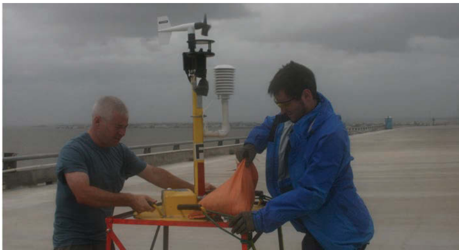
Josh Wurman and a technician deploy a rugged quickly deployable instrumented 'Pod' as Hurricane Ike approaches Galveston, Texas
