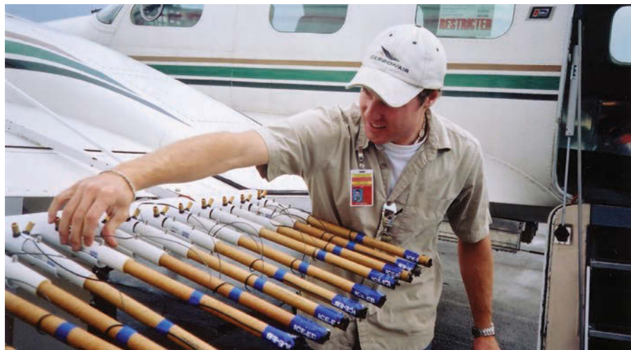
Replacing aileron AgI flares after a hail suppression mission in Alberta. Each flare burns for six minutes. Photo by Daryl O'Dowd
