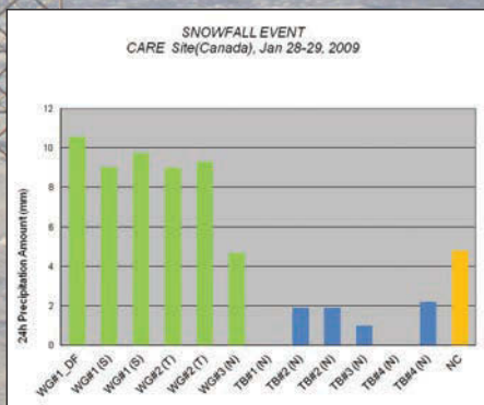
The accumulated precipitation amount over 24 hours reported from different automatic gauges and configurations are influenced by the precipitation type. Results from the Canadian Centre for Atmospheric Research Experiments (CARE). (WG – weighing gauges; TB – tipping bucket type gauges, DF (DFIR) double-fence intercomparison reference shield, S for single-Alter shield, T for Tretyakov shield, U for unshielded, and NC for a non-catchment type sensor (optical forward scatter))
