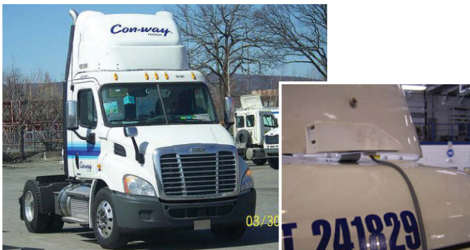
Weather instrumentation mounted on vehicle cab
