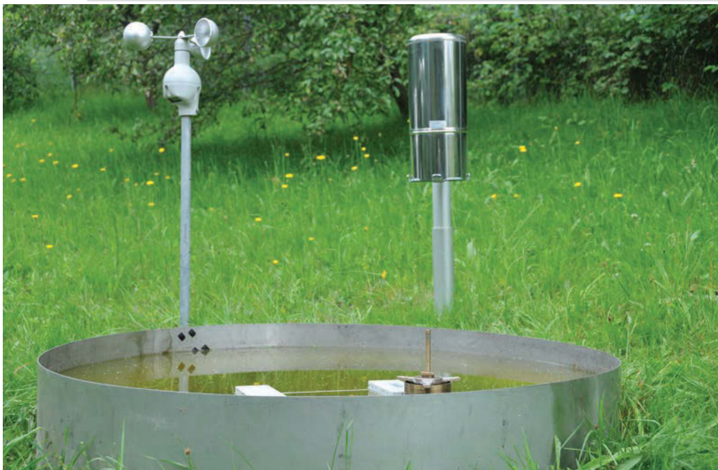
Example of a Class A evaporation pan with micro-meter, floating thermometer and anemometer with a manual rain gauge
