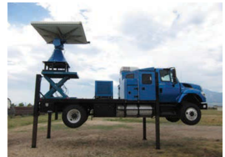
The Rapid-Scan DOW can collect volumetric data in tornadoes, hurricanes, and other severe weather with updates every seven seconds
